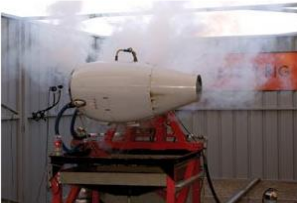
Figure 10 – Engine nacelle suppression test [38]
