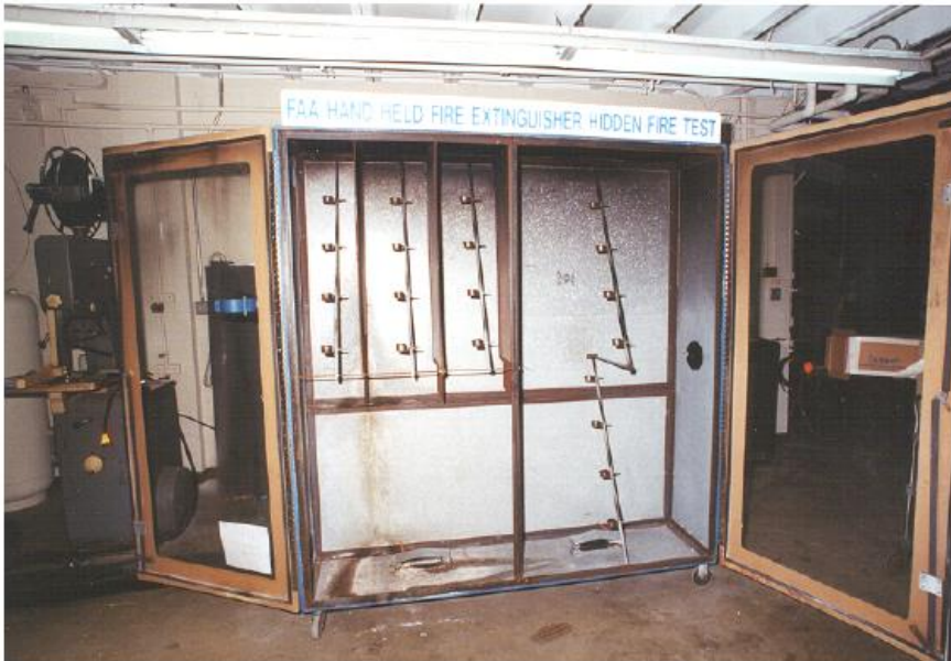
Figure 16 – Hidden fire flooding test [47]
