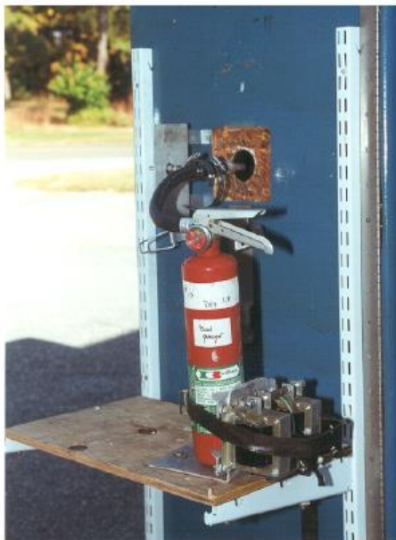
Figure 17 – Hidden fire test extinguisher [47]
